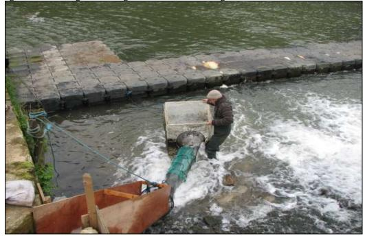
Figure 3: photograph illustrating the chute and holding box.
