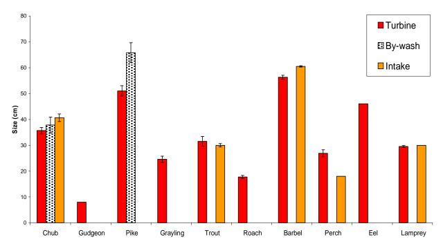
Figure 4: The average size (+/- one standard error) of fish of various species either passing down the turbine or by-wash or remaining in the intake area upstream of the turbine
